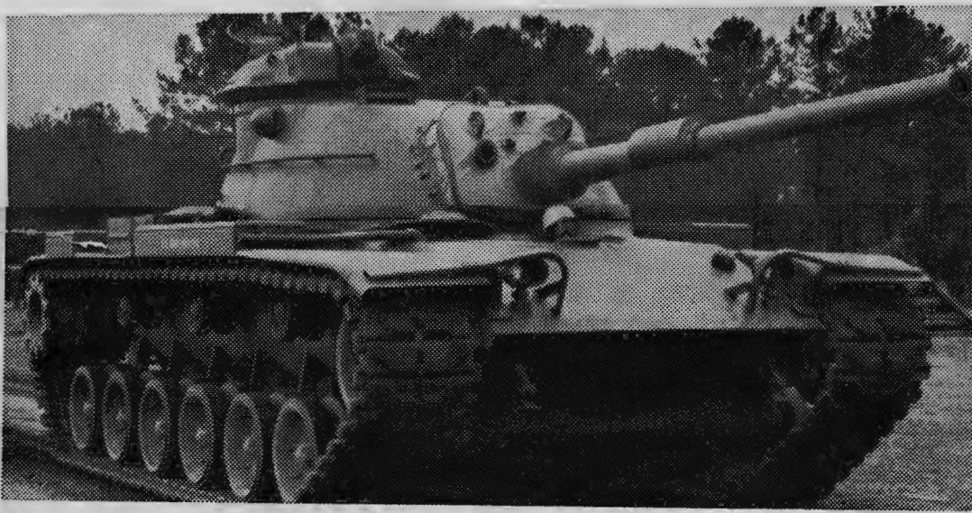
M-60 TANK — The Army's new M-60 tank, which carries a four-man crew, is armed with a high velocity 105mm gun mounted in a turret which turns 360 degrees under hydraulic power. It is also armed with 50 cal. and 7.62mm machine guns plus two 45 cal. sub-machine guns.
