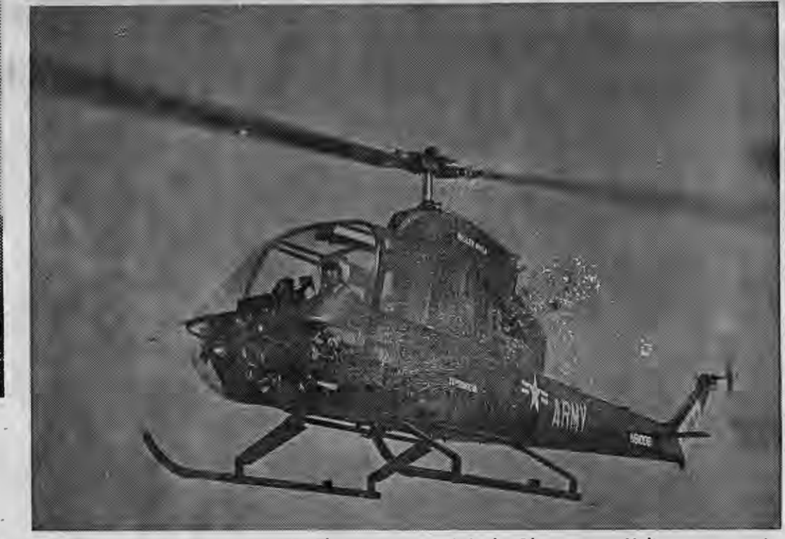
TURBINE-POWERED HELICOPTER —This new OH-5A Light Observation Helicopter, now in production, is fitted with an automatically-stabilized rotor system. It is powered by the Allison T63 gas turbine engine, with speed 50 per cent higher than the present light helicopter in use.
