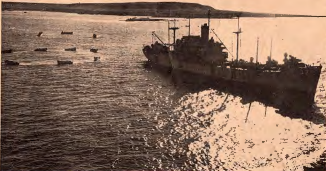
AWAIT ORDERS - LCVPs circle alongside the USS Cavalier (APA 37) awaiting orders to come alongside and load troops. LCVPs are used primarily to land troops on assault beaches. They are the smallest and most numerous of the landing craft family.
