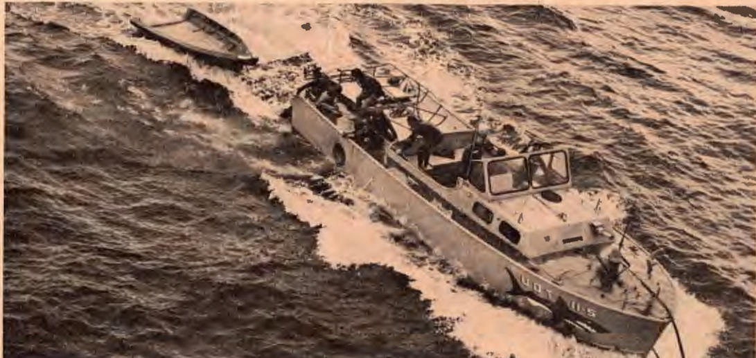
RECOVERY BOAT - A recovery boat from Underwater Demolition Team 11 demonstrates a new pickup system employed in recovering frogmen from the water off enemy held beaches. At high speed, the boat picks up a floating line connecting two fiberglass sleds with UDT swimmers, and a winch rapidly pulls the sleds and men up to the boat's stern.
