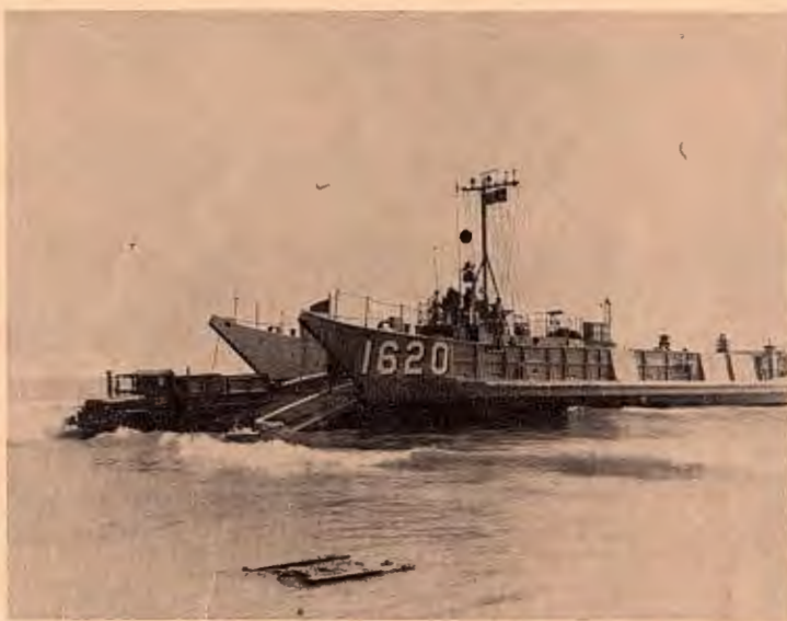
LEFT - The LCU 1620 (landing craft utility) is one of the newest and largest members of the Navy's family of ships. She is a unit of Assault Craft Squadron One. The LCU's primary wartime function is to land heavy vehicles (tanks), equipment and cargo on the beach in an amphibious assault.
