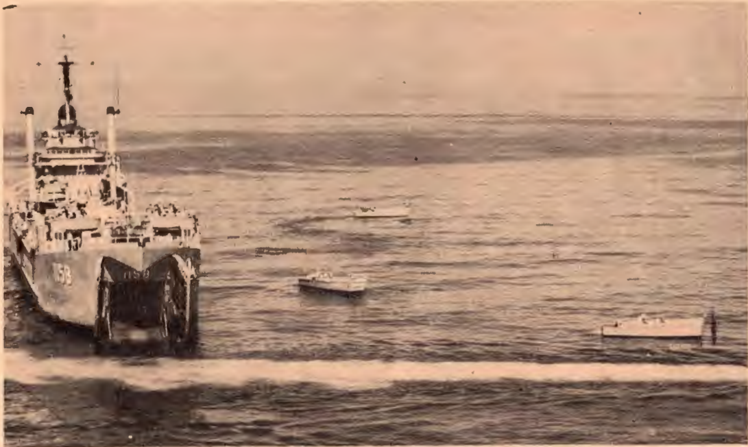
USS TIOGA COUNTY - The Tioga County (LST 1158), the flagship of Landing Squadron Three, lies at anchor off an assault beach performing the duties of a boat lane control vessel. Circling alongside her are three of the four LCVPs (landing craft vehicle personnel) she is equipped to carry.
